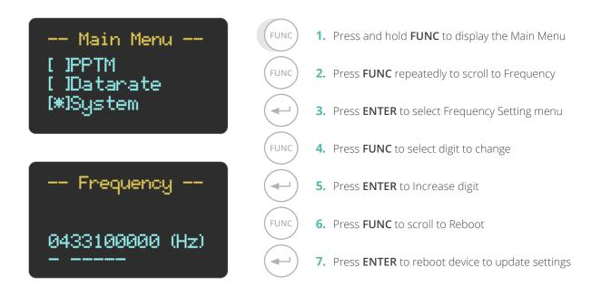
Modules must be on the same frequency to communicate with each other
